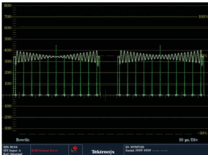
Figure 73. Bowtie display Pr gain error vs. Y.
