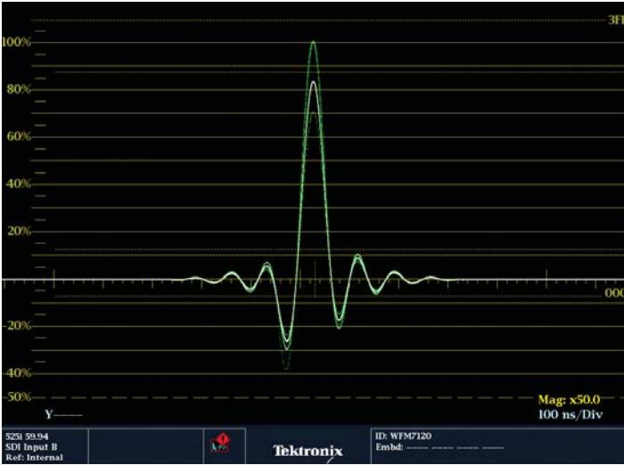
Figure 28. 270 Mb/s EAV timing reference packet viewed as an analog luma channel signal.
