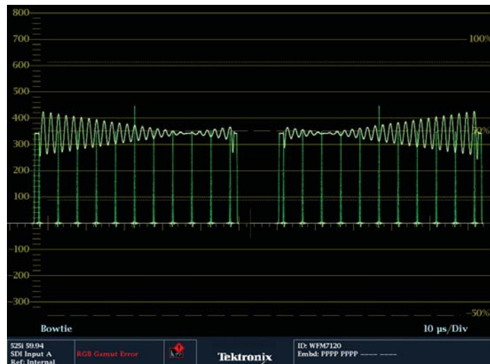
Figure 72. Bowtie display, Pb delayed 55ns, Pr advanced 50ns Y.
